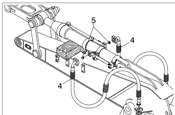
Sling bucket cylinder assembly(8) and remove bolt(6) then pull out pin (5).
