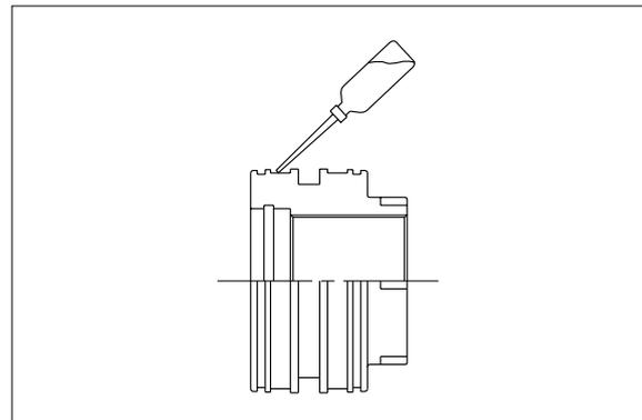
Fit piston seal(17) to piston.
