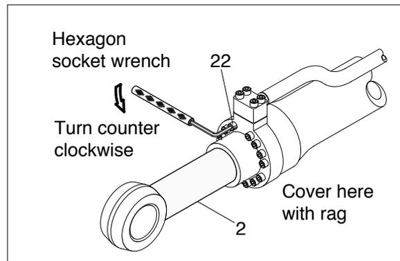
Draw out cylinder head and rod assembly together from tube assembly(1).
