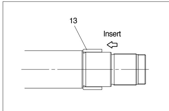
Fit piston assembly to rod assembly.
