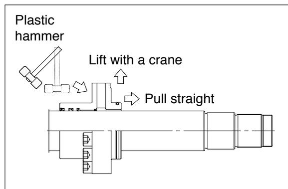
**(3) Disassemble the piston assembly**
