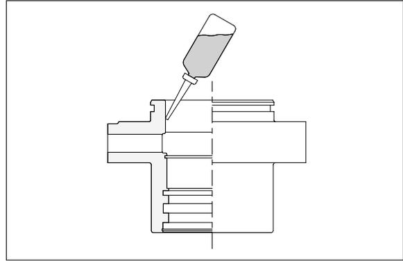
Coat dust wiper(9) with grease and fit dust wiper(9) to the bottom of the hole of dust seal.
