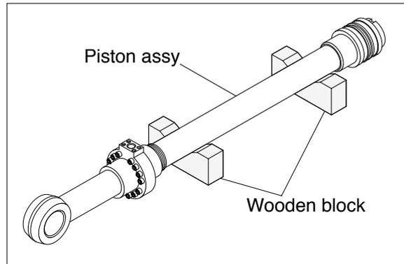
**(2) Remove piston and cylinder head**
