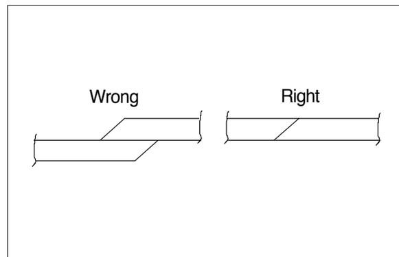
Rod seal(6) has its own fitting direction. Therefore, confirm it before fitting them. Fitting rod seal(6) upside down may damage its lip. Therefore check the correct direction that is shown in fig.
