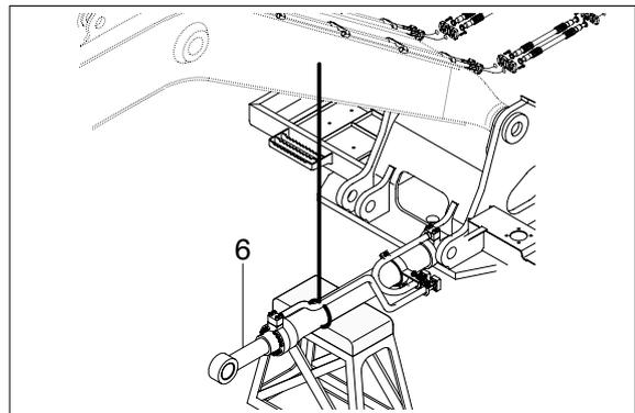
Disconnect boom cylinder hoses(7) and put plugs on cylinder pipe.
