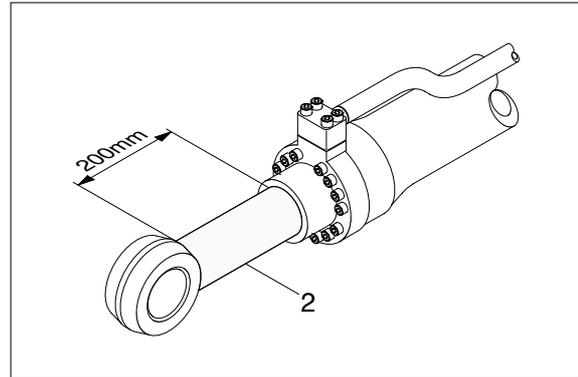
Loosen and remove socket bolts(22) of the gland in sequence.
