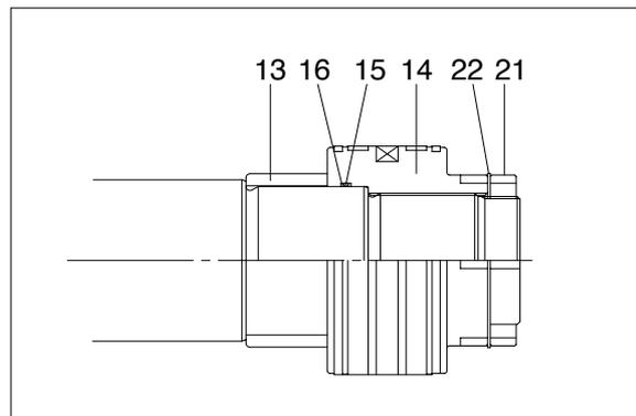
Remove the cylinder head assembly from rod assembly(2).
